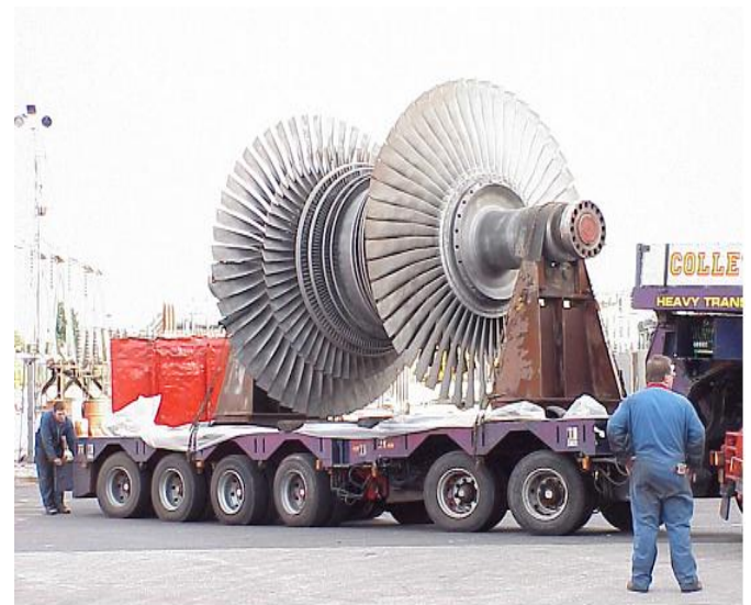
Figure 2: A low pressure steam turbine that makes one of 5 turbines on a generating unit
