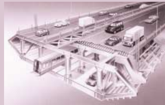
Tsing Ma's innovative streamlined vented two-level deck designed to withstand typhoon winds
