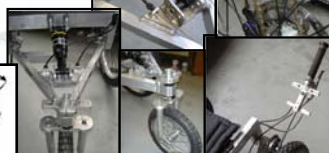
MANUFACTURE OF FULLY OPERATIONAL PROTOTYPE FEATURING ALUMINIUM CONSTRUCTION, AIR SHOCKS, DISC BRAKES, CHAIN DRIVE, CABLE STEERING
