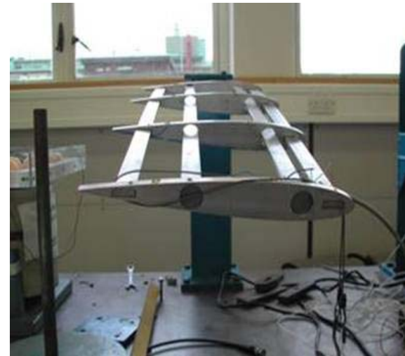
Internal Model Wing Structure Showing Rotating Spars
