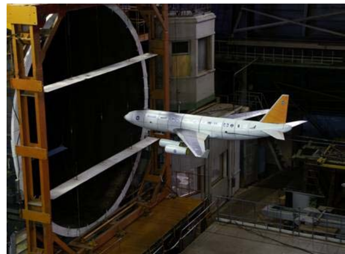
EuRAM Model With Adaptive All-Moving Tail
