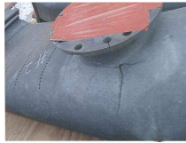
Photograph of damaged gas turbine piece courtesy of F. C. Iannoun
